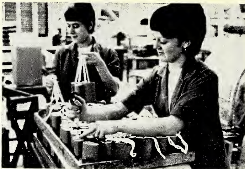
Soap, in every shape and form, is one of the most successful commodities sold as Christmas presents each year—and soap-on-a-rope is a current favourite. The girls pictured here are working at the Yardley factory putting the rope into Sea Jade soap before it is stamped into the familiar shapes of Seahorses and Cougar squares
